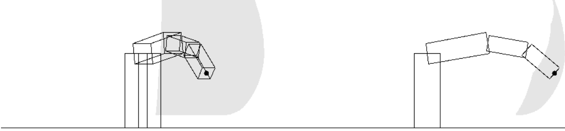
Figure 14: Rule found by VI-Analysis. The robot arm illustrates a configuration which is classified as being SAFE. The grey-shaded area indicates the preimage of the generalized rule. This region, too, will be predicted as being SAFE by the network. (a) Front view. (b) Two-dimensional side view (including a slice of the rule).
