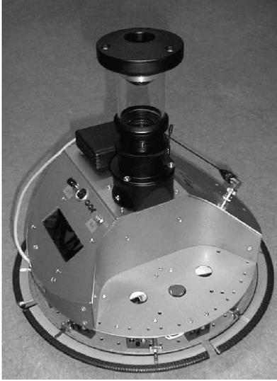
Figure 7: The Samurai robot, equipped with an omnidirectional camera and a magnetic compass.
