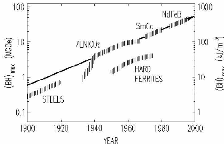
Figure 1. Improvements in  $((\text{BH})_{\text{max}}$  for permanent magnets since 1900.
