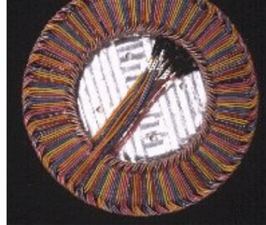
Figure 4b. Stator winding for Aurora solar car.
