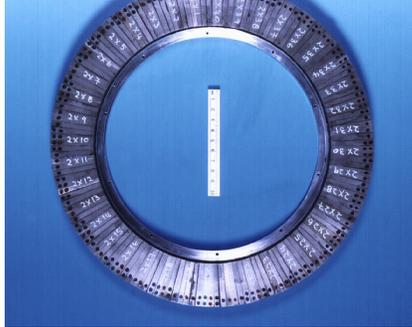
Figure 4a. Magnet ring for Aurora solar car motor.
