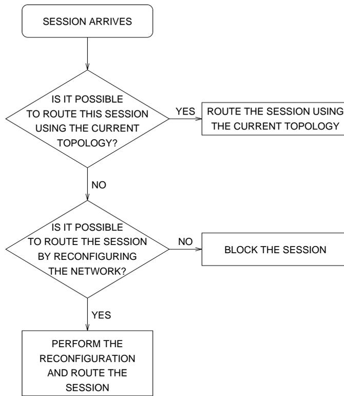
Figure 5: Dynamic operation of the WDM Reconfigurable Network
