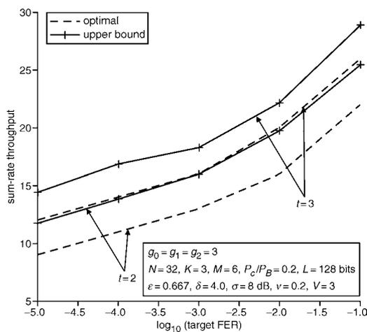
**Fig. 1** Comparison between optimal sum-rate throughput and upper bound on sum-rate throughput
