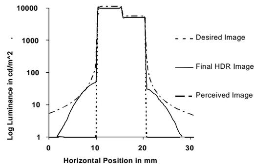
**Figure 4. Comparison of display and eye introduced blur at a contrast boundaries of 0cd/m<sup>2</sup> to 10,000cd/m<sup>2</sup>, 10,000cd/m<sup>2</sup> to 5,000cd/m<sup>2</sup> and 5,000cd/m<sup>2</sup> to 1cd/m<sup>2</sup>.**
