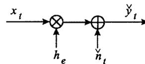
Fig. 1. Equivalent channel model for space–time block codes and linear combining at the receiver.
