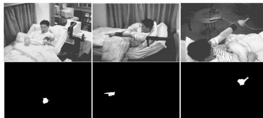
Figure 10 Three Images from Each Camera and Detected Hand Region
