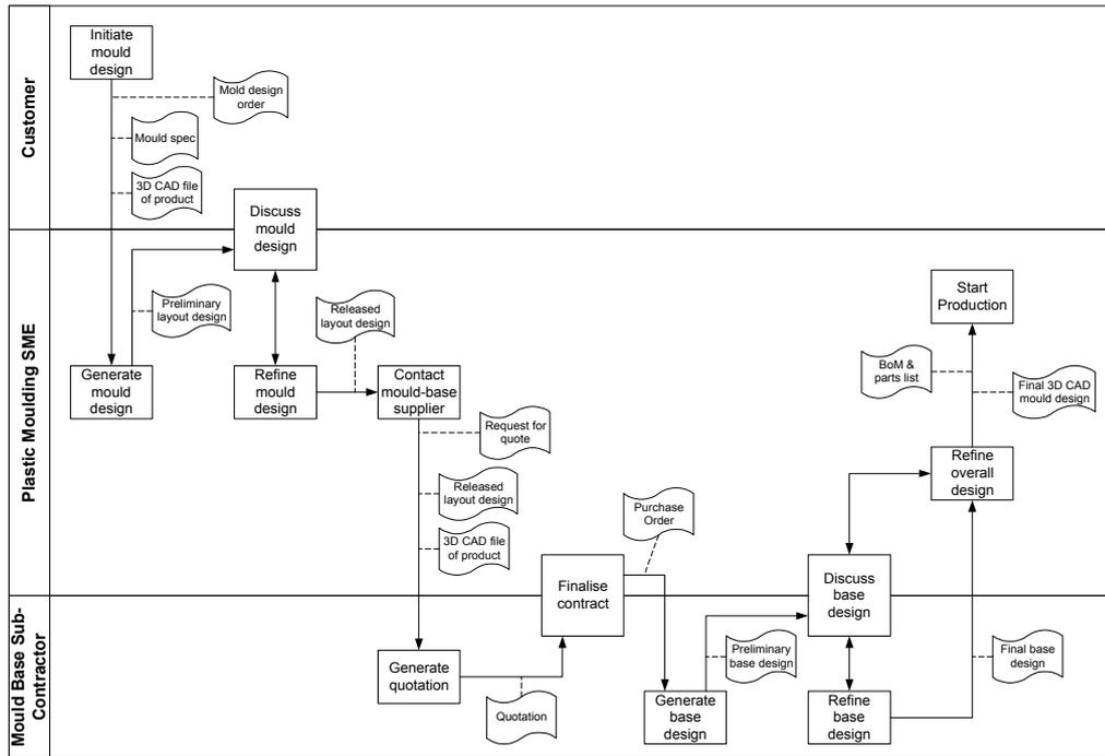
Fig. 2. Design chain for a plastic moulding SME.
