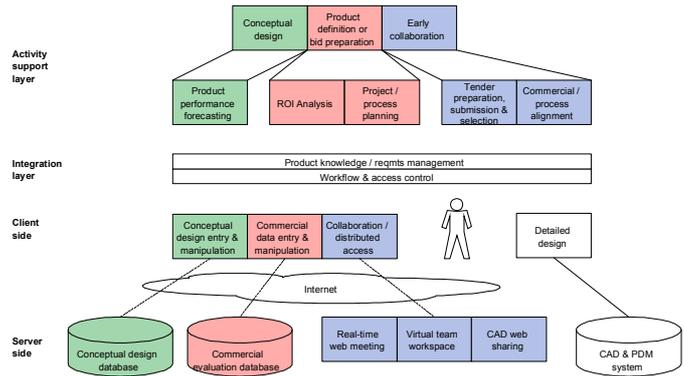
Fig. 3. System architecture for a Collaborative Product Conceptualization & Bidding System (CoProBid).
