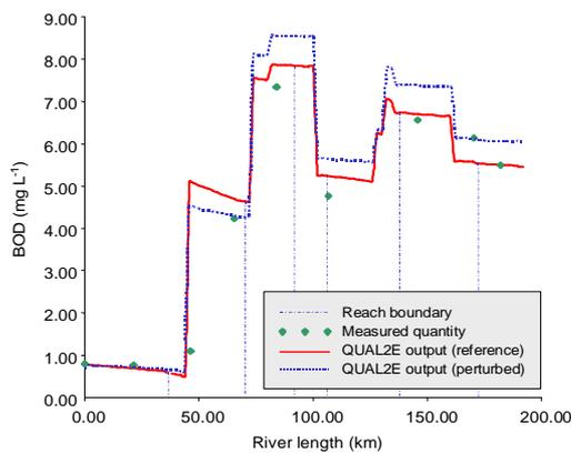
Fig. 5. BOD model output in the reference and perturbed Summer scenario, together with the calibration data.
