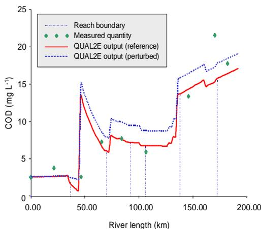
Fig. 6. COD model output in the reference and perturbed summer scenario, together with the calibration data.
