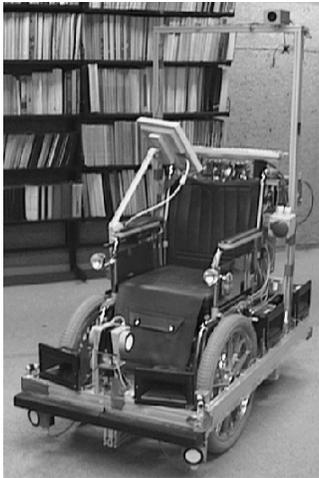
**Fig. 6.** The Bremen Autonomous Wheelchair.
