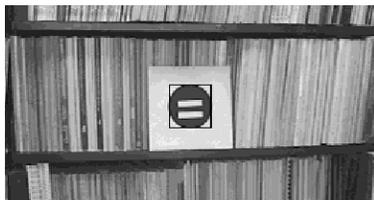
**Fig. 11.** View of an artificial routemark. The square indicates recognition.
