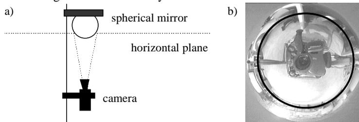
**Fig. 9.** Apparatus for taking panoramic images. a) Scheme. b) Image on the sphere. The circle indicates the mapping region of the horizontal plane.
