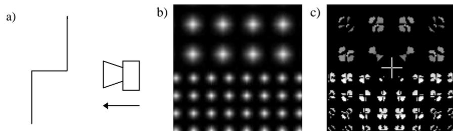
**Fig. 14.** A simulated camera approaching a distance step. a) Scheme of set-up. b) Camera view. c) Estimated depth coded as brightness. Brighter areas correspond to farther surfaces.
