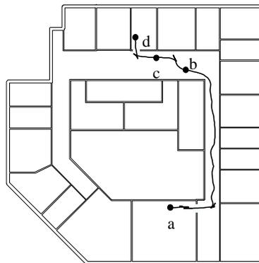
**Fig. 12.** A measured trajectory that has been generated by the combination of four basic behaviours. a) Follow left wall. b) Follow right wall. c) Turn into right door. d) Stop.
