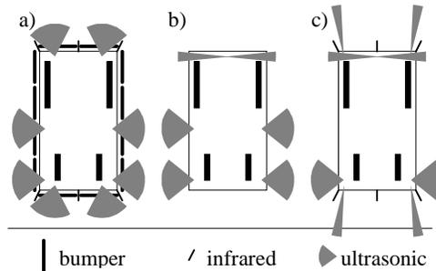
**Fig. 7.** The sensor control subsystems. a) Collision detection. b) Steering restriction. c) Navigation.
