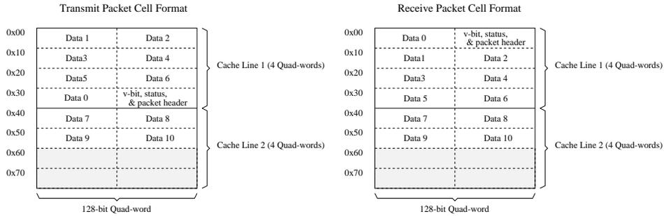
Figure 3: Transmit cell and receive cell packet formats.
