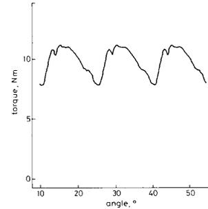
Figure 4. Torque/angle for conventional chopping waveform
