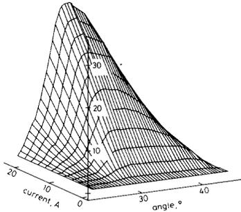
Figure 2. Torque (Nm) vs. current and angle
