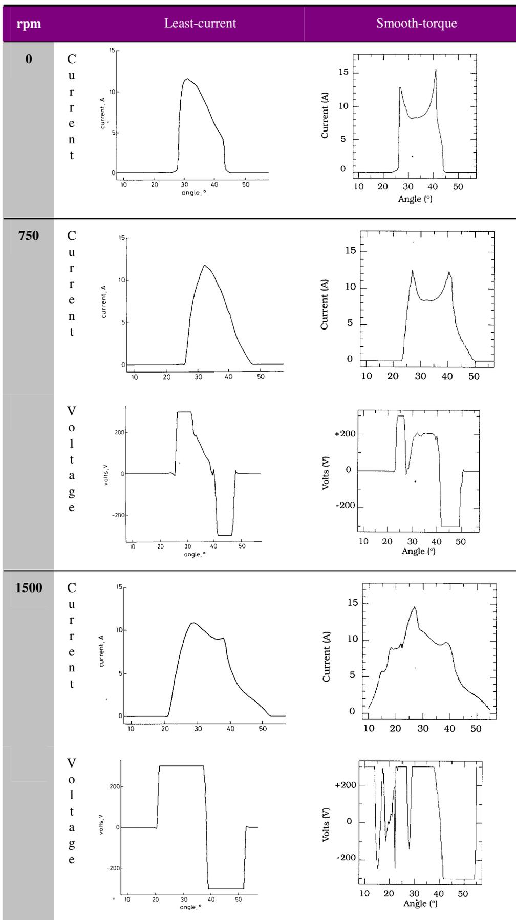
Figure 5. Optimised current waveforms and associated voltage waveform
