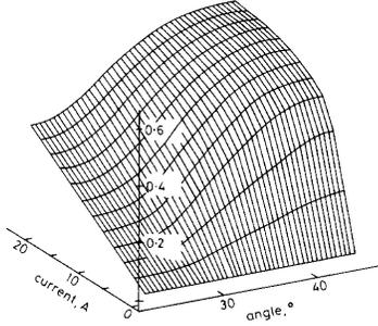
Figure 1. Flux linkage (Wb) vs. current and angle
