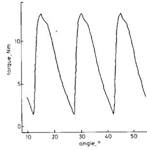
Figure 3. Torque/angle for least-current, 0 rpm, waveform
