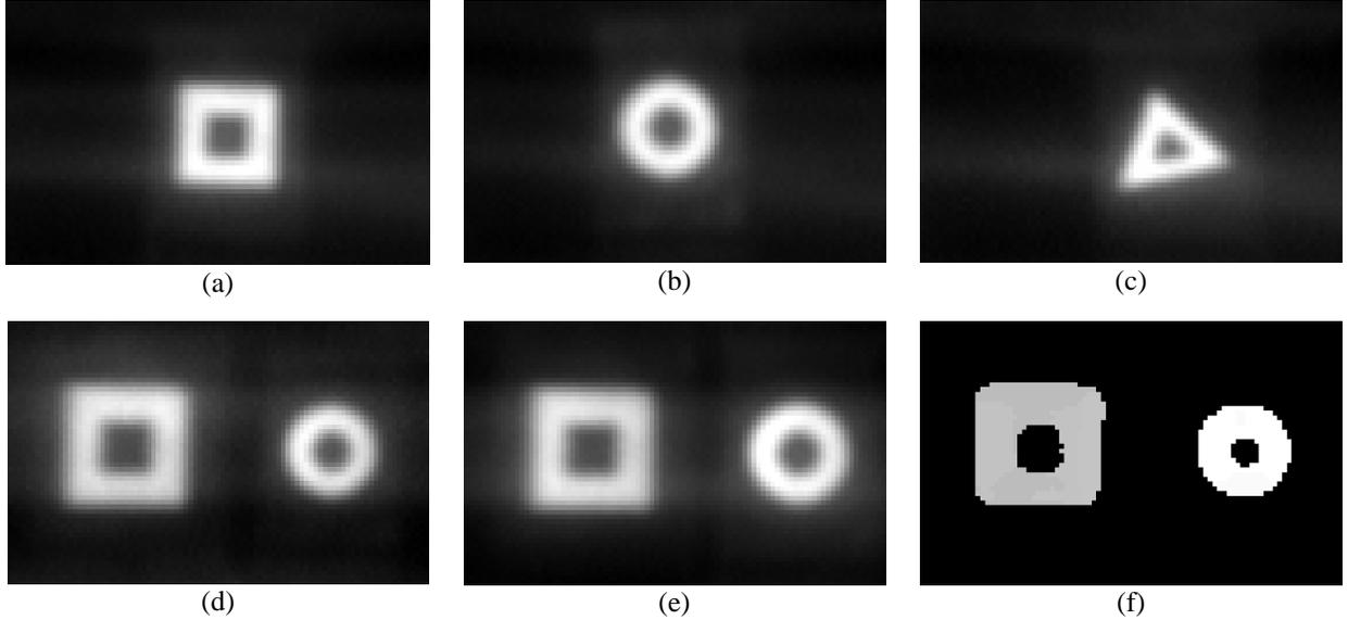
Fig. 4: Views of the 3D objects used in the experiments – (a), (b) and (c) are planar reference objects – (d) and (e) are composite 3D input scenes with the reference objects at various distances – (f) Map of the estimated depths for the 3D scene shown in (d).
