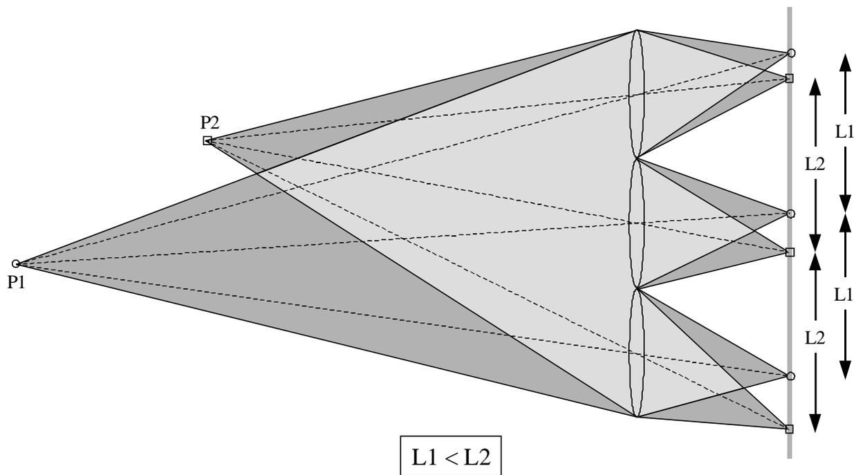
Fig. 2: Image formation through the microlens array.
