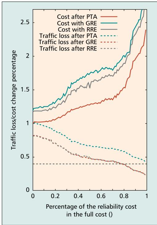
■ **Figure 6.** Network cost and traffic loss using different parameters, comparing RRE.
