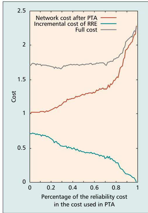
■ **Figure 7.** Network and expansion cost with fixed  $L_{lim}$  and variable  $\alpha$  parameter.
