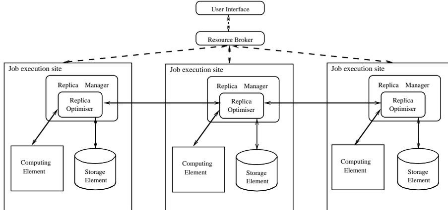
Figure 1: Simulated DataGrid Architecture.
