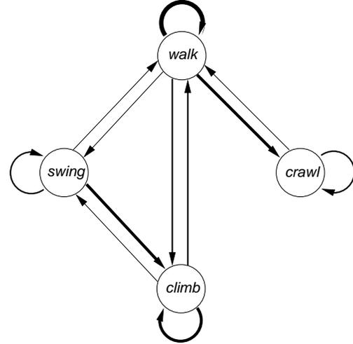
**Figure 8:** The locomotion mode finite state machine
