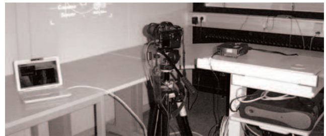
Figure 1. The optical triangulation devices.
