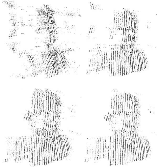
Figure 8. Point cloud without (top) and with (bottom) white background plane and artifact elimination for \alpha = 90^\circ (left) and \alpha = 60^\circ (right).
