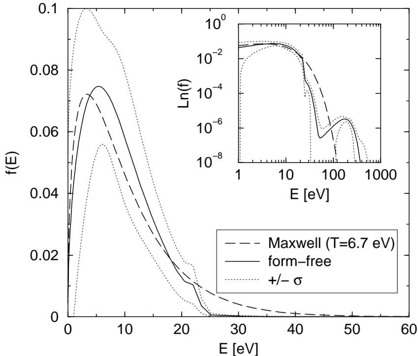
*Figure 3.* The dashed line depicts a Maxwell distribution of the temperature measured with the Langmuir probe. The solid line shows the form-free estimation of the EED with the adaptive-kernel approach. The steep decrease at an energy of about 20 eV arises due to a loss channel by excitation of helium. The peak at about 100-200 eV is interpreted as an accumulation of high energy electrons due to the heating mechanism.
