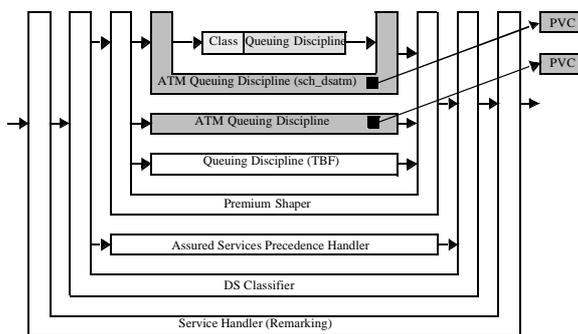
**Fig. 7** DiffServ Implementation with ATM Queuing Discipline for EF
