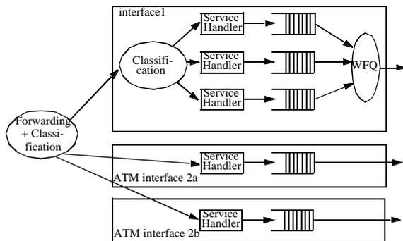
**Fig. 5** DiffServ Implementation over ATM I
