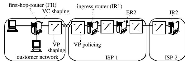
Fig. 3 DiffServ over ATM with VP aggregation
