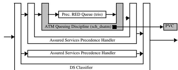
**Fig. 9:** DiffServ Implementation with ATM Queuing Discipline for AF
