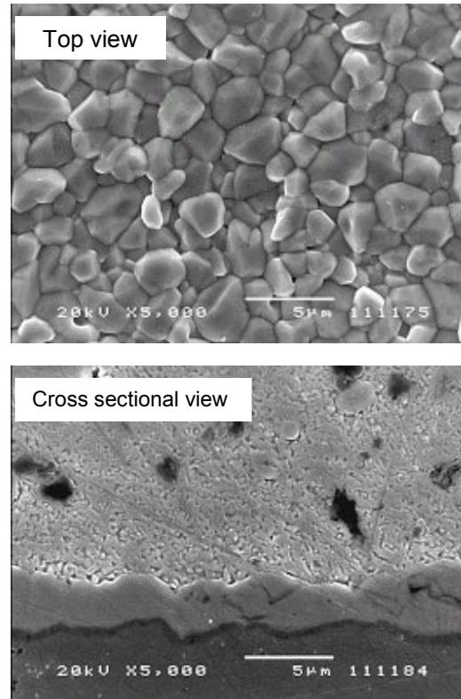
Fig. 3. Top and cross sectional views of the IMCs formed between Sn3.5Ag and Ni-P UBM after 100 hours aging at 170°C.
