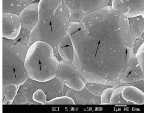
Fig. 8. Small grains merge themselves into larger grains (SnAg solder with Ni-P UBM, annealed at 190°C for 100 h. Arrows indicate the merging path of adjacent grains).
