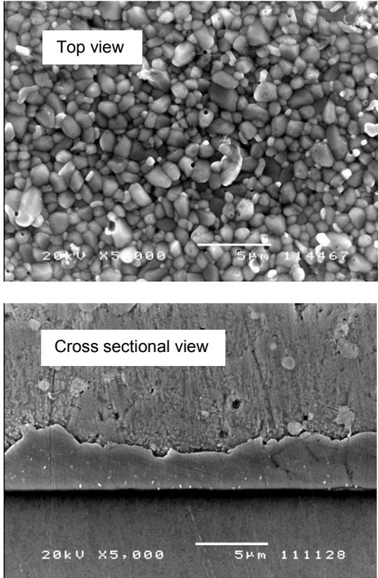
Fig. 5. Top view of the  $Ni_3Sn_4$  of in the Sn3.5Ag vs sputtered nickel UBM system, after aging at 190°C for 400 hours.
