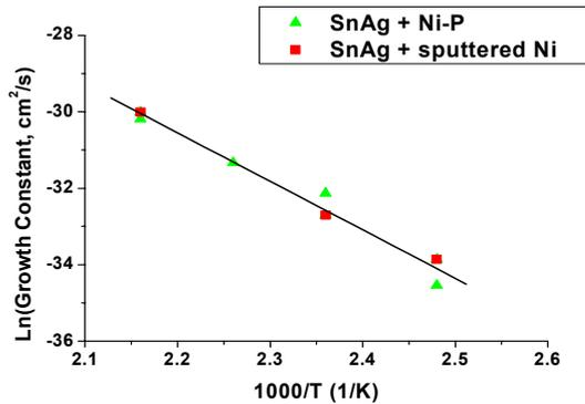
Fig. 9. Arrhenius plot for the formation of IMC between SnAg3.5 solder and Ni-P and pure Ni UBMs.
