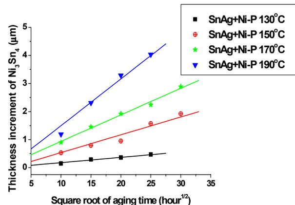
Fig. 4. Linear correlation of the IMC growth with square root of thermal aging time.
