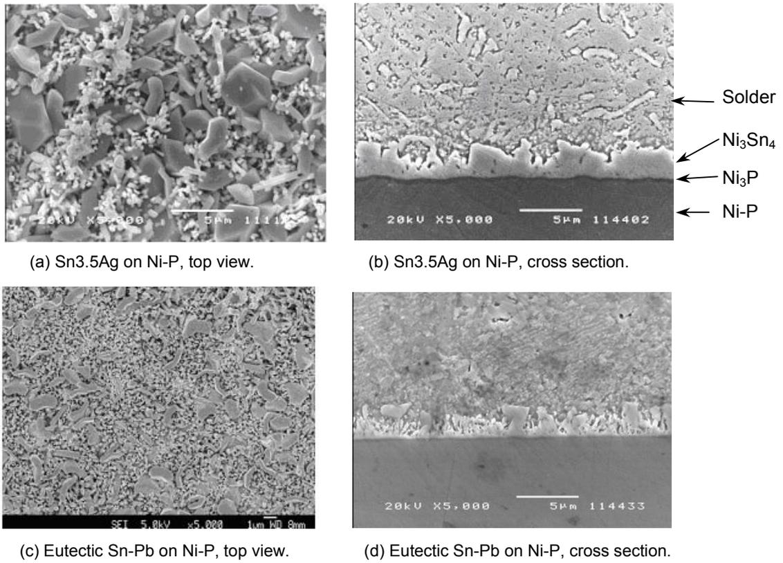
Fig. 1. Top and cross sectional views of the intermetallic compounds formed between Sn3.5Ag and eutectic Sn-Pb solders and electroless Ni-P alloy UBM.
