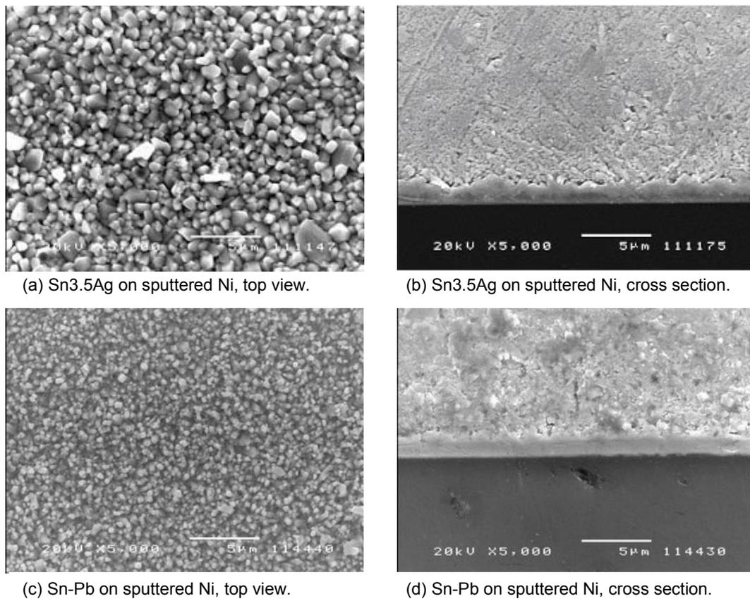
Fig. 2. Top and cross sectional views of the intermetallic compounds formed between Sn3.5Ag and eutectic Sn-Pb solders and sputtered nickel UBM after reflow.
