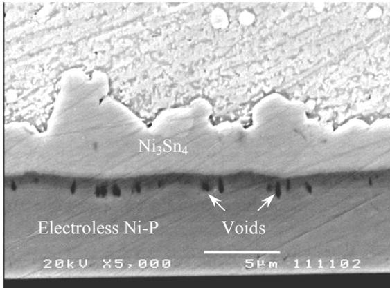
Fig. 7. Voids at the interface between Ni<sub>3</sub>P and Ni-P UBM.
