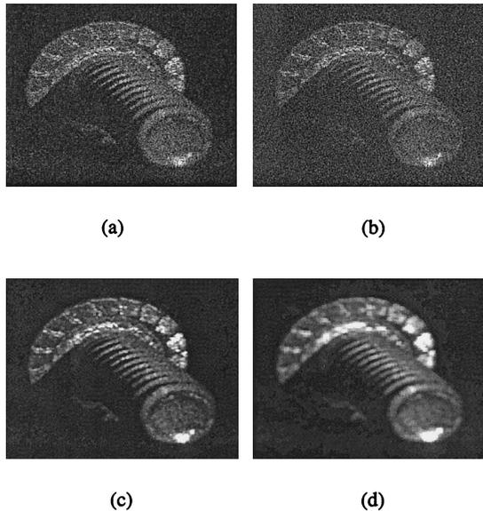
Fig. 3. Numerically reconstructed 3D objects of a screw from (a) a fully complex field, (b) phase-only information, (c) low-pass filtered 3D objects with a mean filter of  $11 \times 11$  pixels, (d)  $21 \times 21$  pixels after reconstruction with phase-only information.
