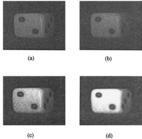
Fig. 2. Numerically reconstructed 3D objects of die from (a) a fully complex field, (b) phase-only information, (c) low-pass filtered 3D objects with a mean filter of  $11 \times 11$  pixels, (d)  $21 \times 21$  pixels after reconstruction with phase-only information.
