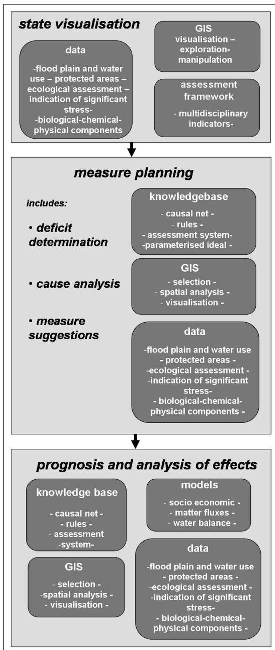
**Figure 5.** Process sequence and relating software components (dark boxes).
