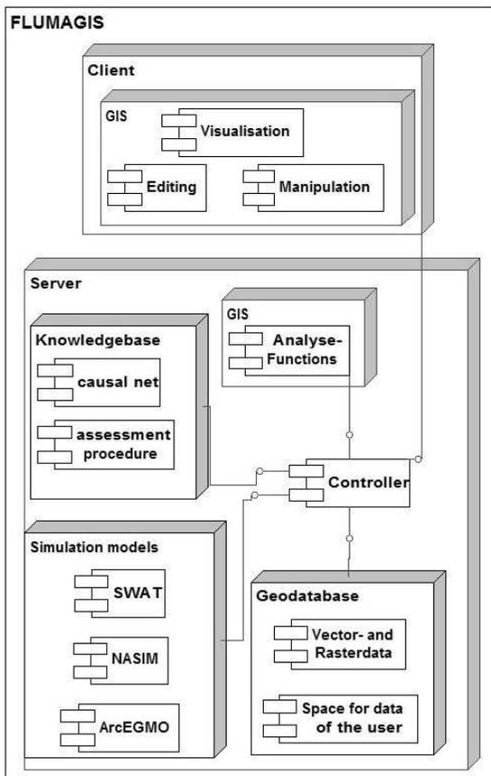
**Figure 3.** FLUMAGIS system architecture.
