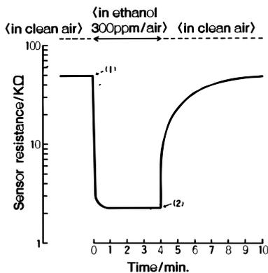
Fig. 1. Typical response of the TGS 822 sensor when the atmosphere changes from clean air to 300ppm ethanol vapor (1), and reverts back to clean air (2)
