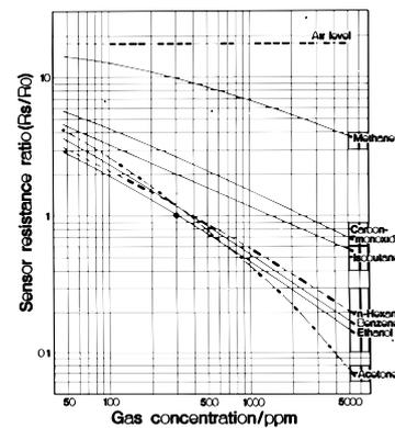
Fig. 2. Sensitivity characteristics of the TGS822 sensor to ethanol vapor and other various gases and vapors. The ordinate is the ratio of the sensor's resistances measured at various concentrations of gases compared to the sensor resistance at 300 ppm ethanol vapor
