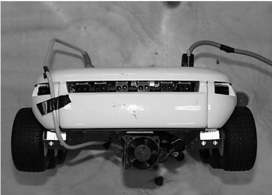
Fig. 4. The front view of the koala robot showing the gas sensing unit placed on the underside.
