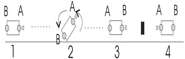
Fig. 5. An example of the localization strategy showing the mobile robot and the two sensors A and B. At 1. Sensor A detects the odor 2. the robot turn 180° and continues to move forward. At 3. the location of the odor is confirmed from the Sensor B's reaction. Finally at 4. the odor is localized by detecting when the robot has past the maximum intensity point.
