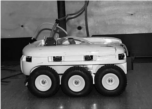
Fig. 3. Side view of the koala robot showing the IR sensors.
