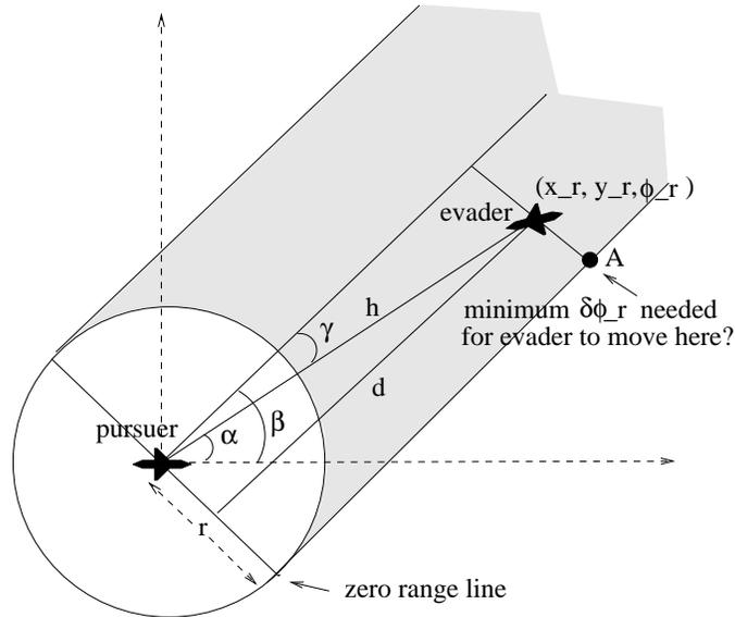
Figure 12: Calculating the minimum deviation angle  $\delta\phi_r$  needed to get out of the unsafe set
