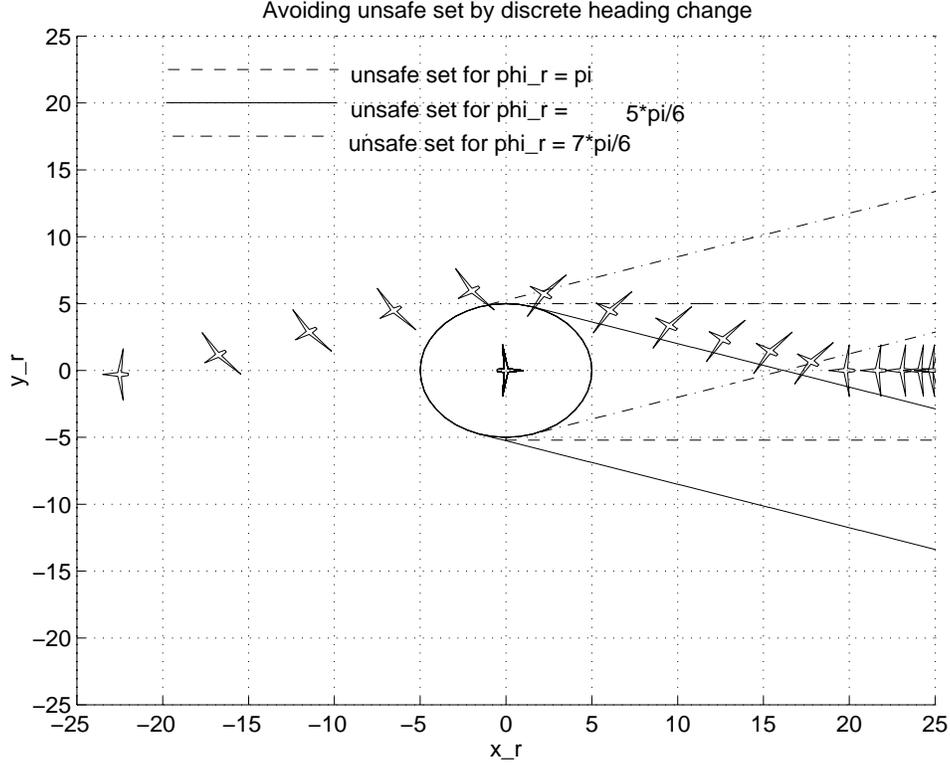
Figure 11: Showing a configuration which is initially unsafe, and the three discrete heading changes which avoid conflict and bring the aircraft back to course
