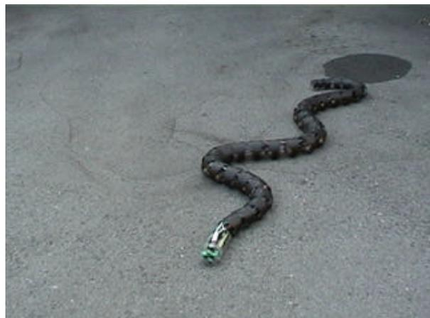
Fig.13: Snake-like robots may be employed to move in narrow spaces, e.g. tracing survivors in collapsed structures
