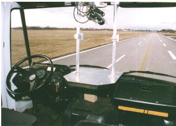
Fig.1: Unmanned car developed by Ernst Dickmanns at UniBW München; field tests with speeds up to 180 km/h, automatic passing of cars, automatic avoidance of potholes, automatic turning into cross-roads
