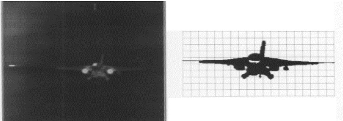
Fig.16: Original infra-red intensity image and extracted aircraft using NRL developed automated technique
