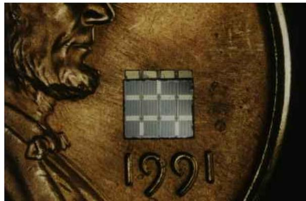
Fig.22: Solar powered chip placed on 1 cent coin, [www.deafblind.com/implant.html](http://www.deafblind.com/implant.html)
