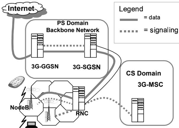
Figure 1: The 3G Network Architecture with an emphasis on the data path. Routing functionality is present in the RNC, the SGSN and the GGSN. [5], [4]
