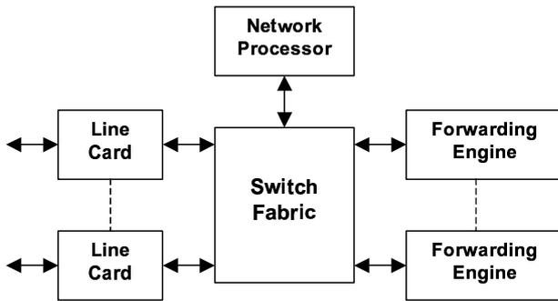
Figure 2: Architecture of a high-speed router [10]
