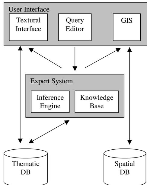
**Figure 1.** Description of system components
