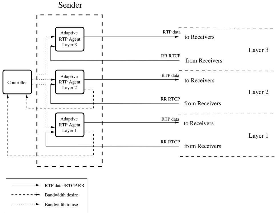
Figure 3: Diagram of the control scheme with three layers
