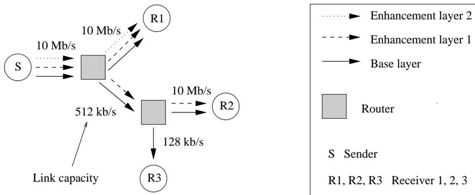
Figure 1: Example of multi-layer transmission
