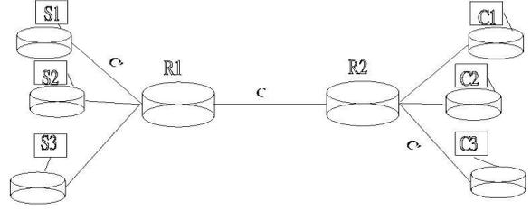
Fig. 1. Simulation setup. Capacities: the core link has  $C=50$ Mbps and the edge links  $C' = 25$ Mbps. Propagation delays: 5msec of the core link and 10msec for the edge links.
