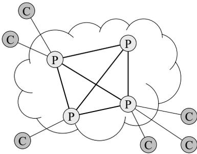
Fig. 1. Illustration of a client/peer system.
