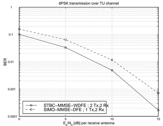
Figure 4: BER vs.  $10 \log_{10}(E_b/N_0)$  for 8PSK transmission over TU channel and (W)DFE (additional receive diversity,  $N_R = 2$ ).
