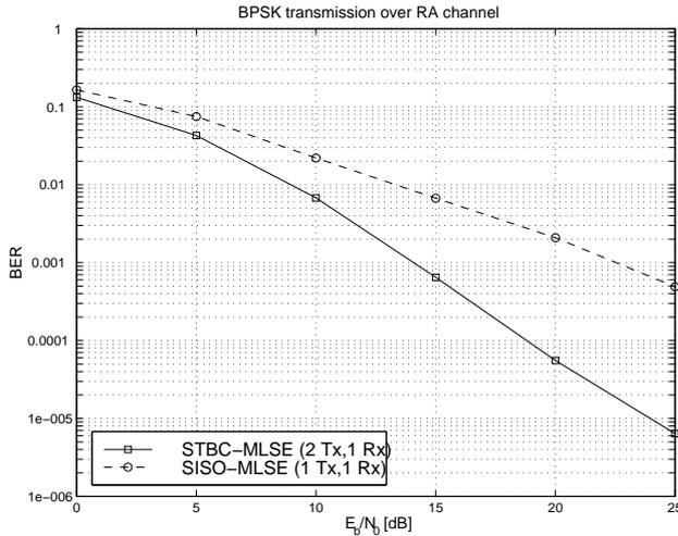
Figure 1: BER vs.  $10 \log_{10}(E_b/N_0)$  for BPSK transmission over RA channel and MLSE ( $N_R = 1$ ). Tx: transmit antenna; Rx: receive antenna.
