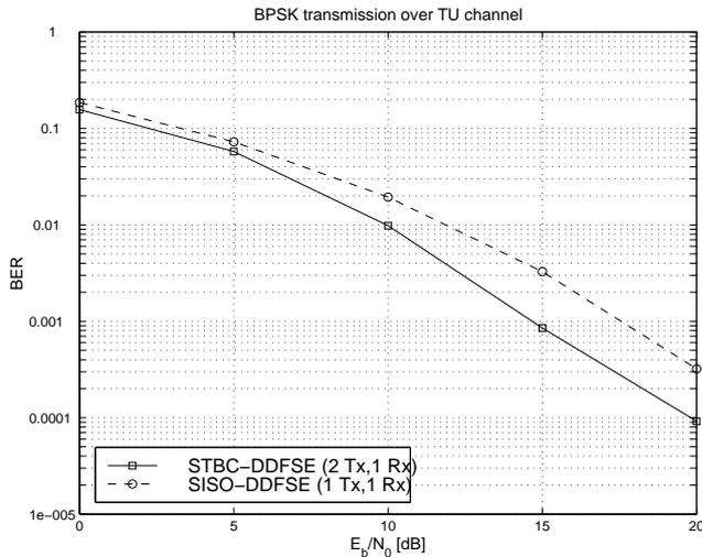
Figure 3: BER vs.  $10 \log_{10}(E_b/N_0)$  for BPSK transmission over TU channel and DDFSE ( $Z = 4$ ) ( $N_R = 1$ ).
