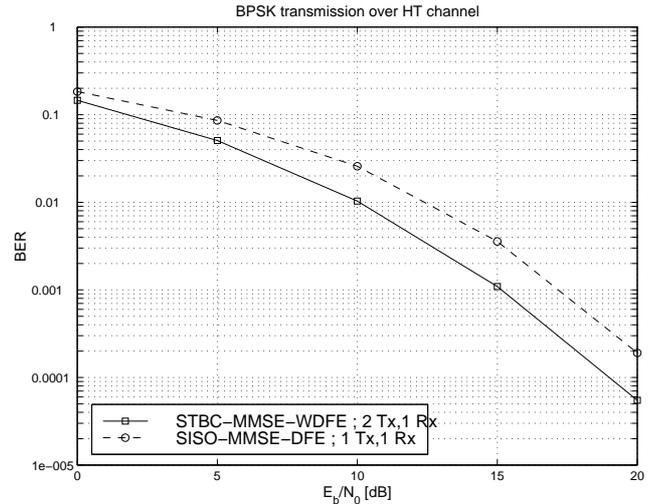
Figure 2: BER vs.  $10 \log_{10}(E_b/N_0)$  for BPSK transmission over HT channel and (W)DFE ( $N_R = 1$ ).
