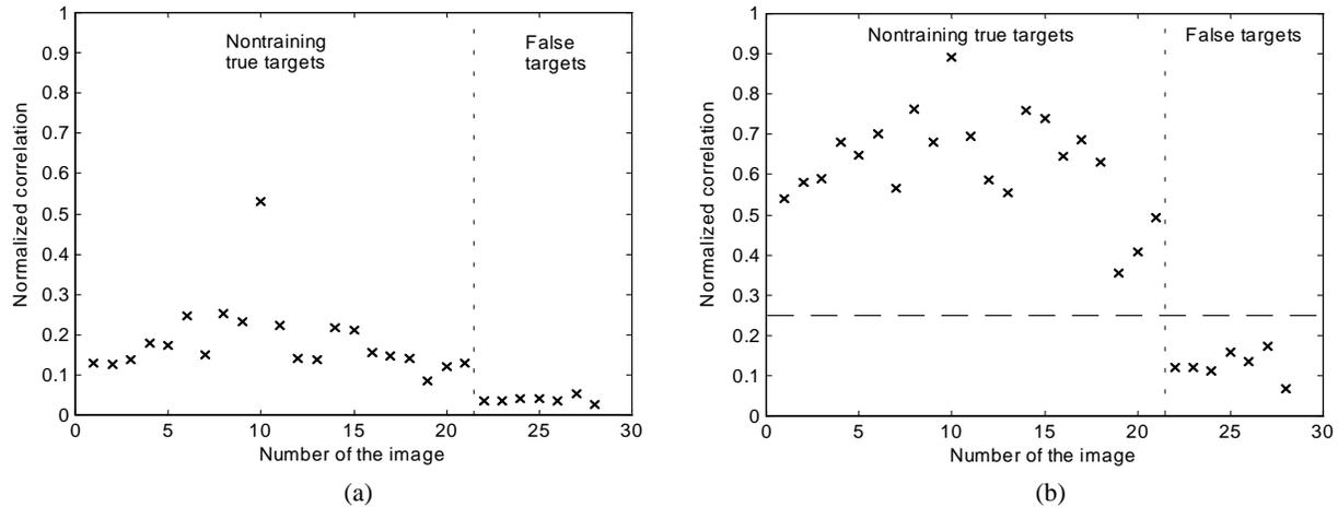
Figure 2. Correlation results with various 3D test objects. (a) Filter made from one single view. (b) Filter made from 15 focused and defocused views based on one single hologram.
