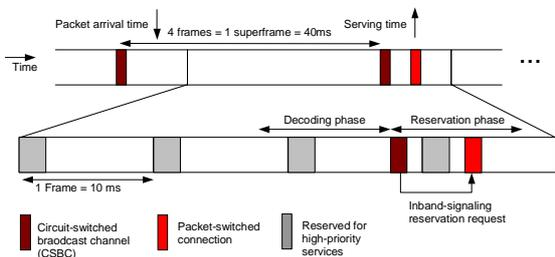
**Figure 1: Reservation of transmit capacity by means of inband-signaling**
