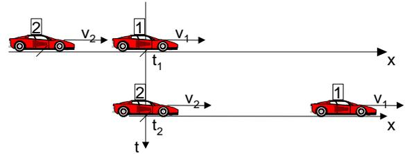
**Figure 2: Derivation of distances between two vehicles based on known time gaps**
