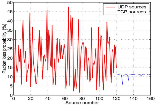
Figure 6: Packet loss probability for each source in mixed UDP/TCP transfer: sources 1 to 120 employ UDP transfers, while sources 121 to 160 employ TCP transfers. Buffer size  $B = 128$  packets and packet size = 552 bytes.
