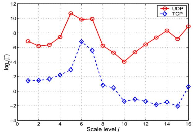
Figure 5: The  $\log_2(\Gamma)$  vs.  $j$  plot of the aggregate traffic arrival process into the router for  $n = 160$  sources, buffer size  $B = 128$  packets, and packet size = 552 bytes.
