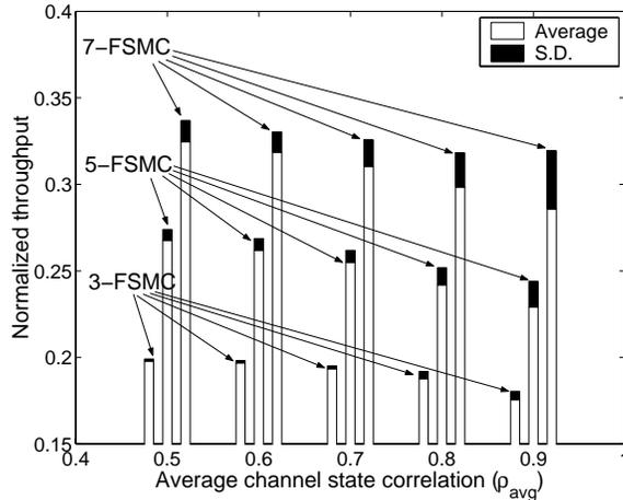
Fig. 2. Average and standard deviation of normalized throughput.
