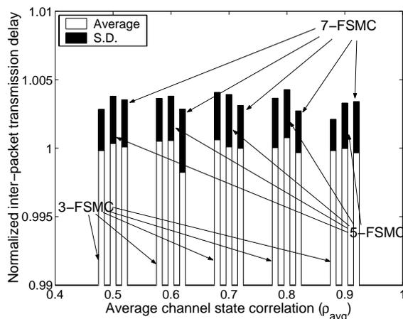
Fig. 3. Average and standard deviation of normalized inter-packet transmission delay.
