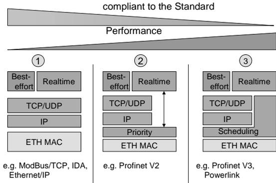
Fig. 4. Structural classification of the different vendor-driven approaches for realtime Ethernet
