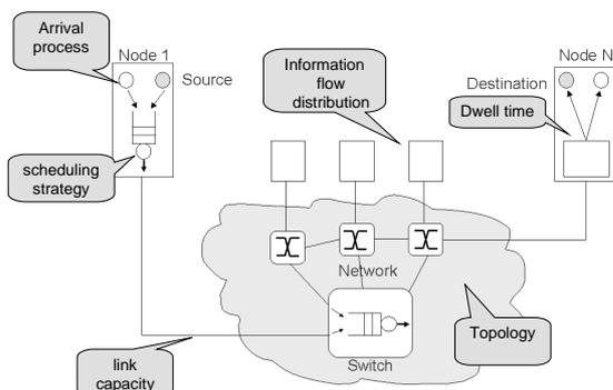
Fig. 2. The various factors, which influence the realtime behavior of a bridged Ethernet system
