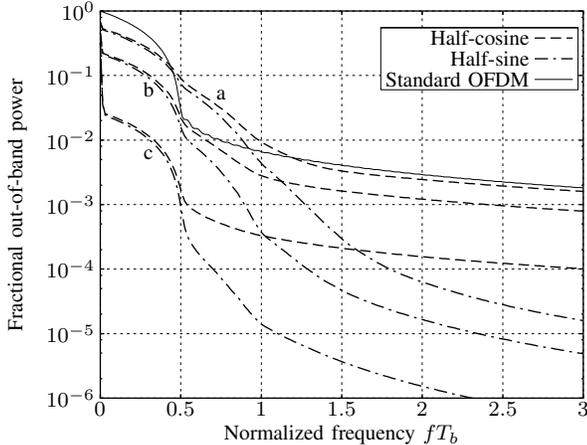
Fig. 4. Fractional out-of-band power for: (a)  $h = 1/2\pi$ , (b)  $h = 0.6/2\pi$ , and (c)  $h = 0.2/2\pi$ .
