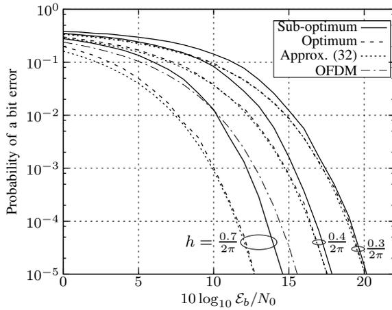
Fig. 12. Comparison of sub-optimum and optimum receiver performance ( $N = 8$ , half-sine subcarriers). The OFDM curve accounts for a 6 dB power gain.
