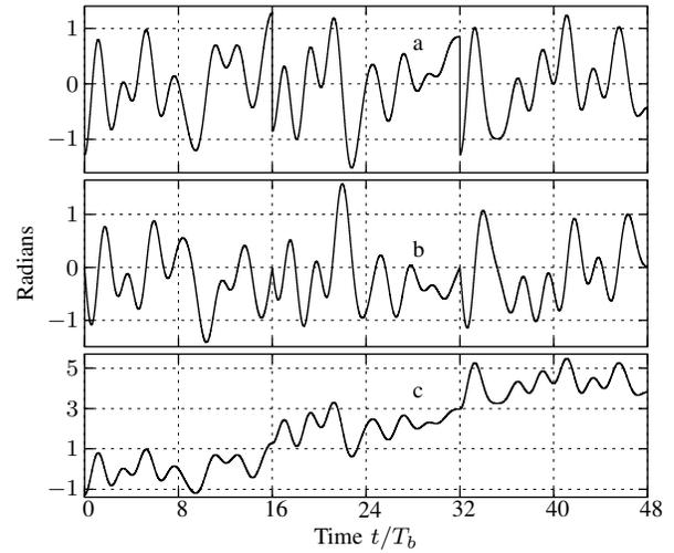
Fig. 1. Generated phase waveform  $\phi(t)$  with  $N = 16$  subcarriers and modulation index  $h = 0.6/2\pi$  for subcarrier types: (a) half-cosine (b) half-sine and (c) half-cosine with memory.
