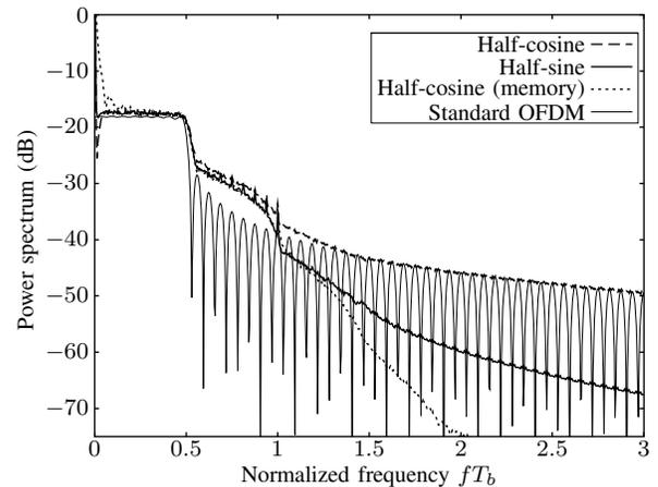
Fig. 2. Power density spectrum for OFDM-PM signals in Fig. 1 compared to standard OFDM.
