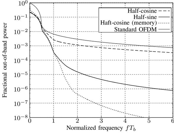
Fig. 3. Fractional out-of-band power curves.
