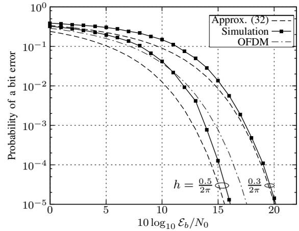
Fig. 11. Simulation results of the sub-optimum OFDM-PM receiver with  $N = 16$  half-sine subcarriers. The OFDM curve accounts for an 8 dB power gain.
