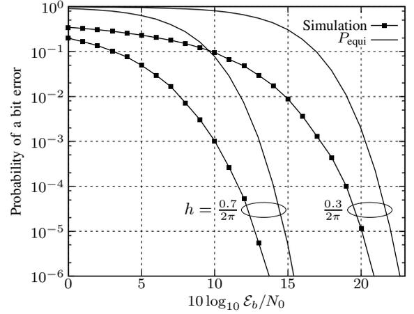
Fig. 9. Probability of a bit error for the optimum OFDM-PM receiver. ( $N = 8$ , half-sine subcarriers)
