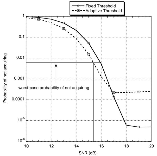
Fig. 6. Acquisition performance averaged over all sequences with worst-case  $P_{nacq} = 0.0051$ . (enlarged x-axis)
