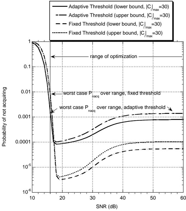
Fig. 1. Acquisition performance for a sequence with maximum autocorrelation sidelobe magnitude of 30 and  $SNR_{min} = 16$  dB.
