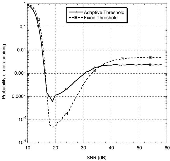
Fig. 4. Acquisition performance averaged over all sequences with  $SNR_{min} = 16$  dB.
