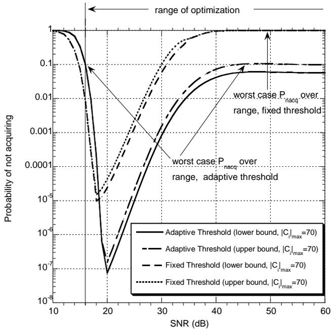
Fig. 3. Acquisition performance for a sequence with maximum autocorrelation sidelobe magnitude of 70 and  $SNR_{min} = 16$  dB.
