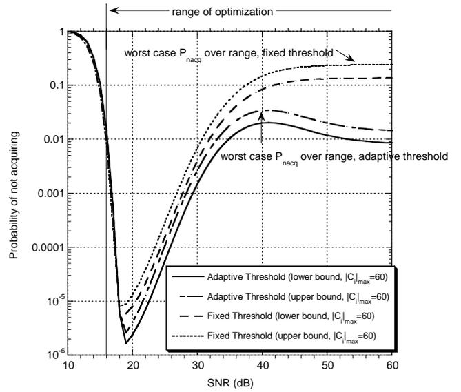
Fig. 2. Acquisition performance for a sequence with maximum autocorrelation sidelobe magnitude of 60 and  $SNR_{min} = 16$  dB.
