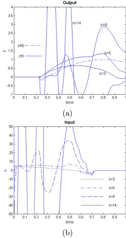
**Figure 1:** The diverged output trajectory and the control input
