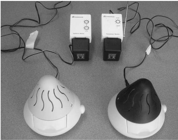
**Figure 2: Scent diffusers and X.10 components used to provide olfactory notification. The diffusers were augmented with directional funnels for efficient scent release.**
