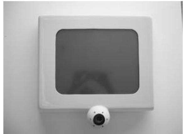
Figure 6. A “transparent” representation for an ubiquitous computing component: a touch-screen enhanced with perceptive capability due to the embedded webcam
