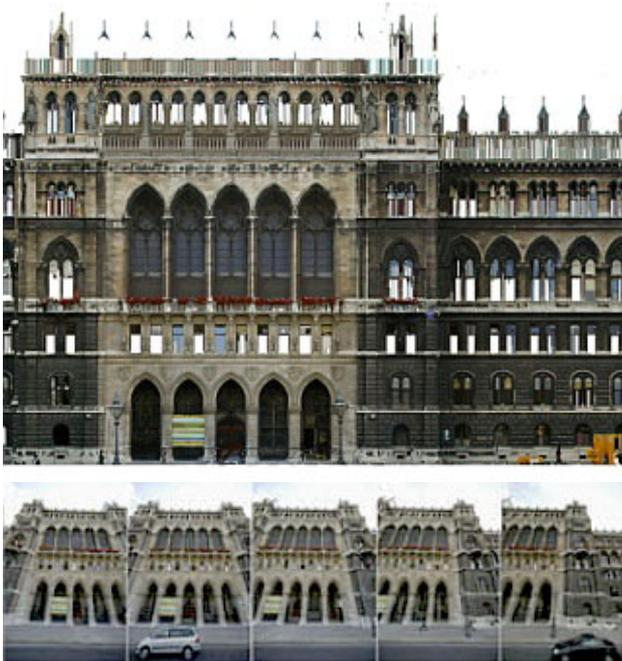
Fig.3: True orthophoto and examples of original images
