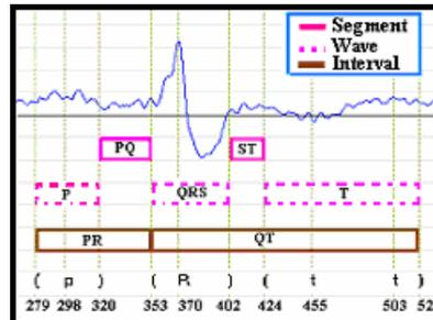
Fig. 7. Waves, segment, interval, limits and peak usually found in a beat
