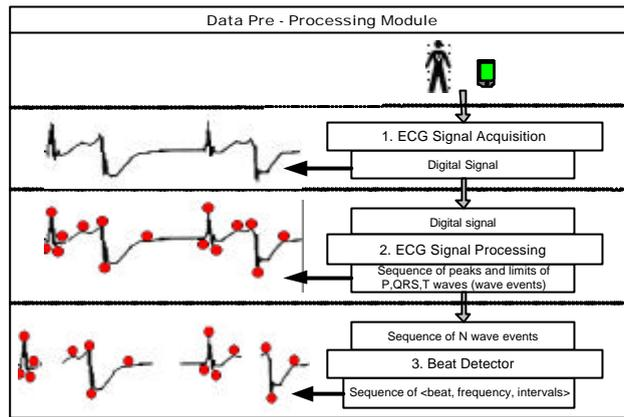
Fig. 3. Data pre-processing module
