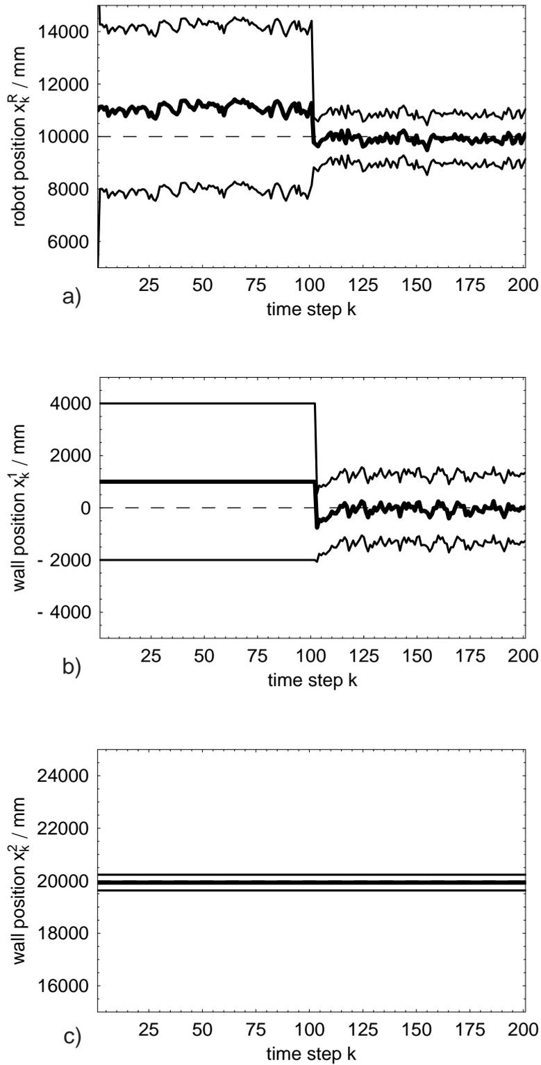
**Figure 4.** Results of applying the Covariance Intersection filter. a) Estimate of robot position. b) Estimate of position of wall 1. c) Estimate of position of wall 2. The figure shows the evolution of the estimated value (thick line) and the evolution of the  $3\sigma$ -bounds.
