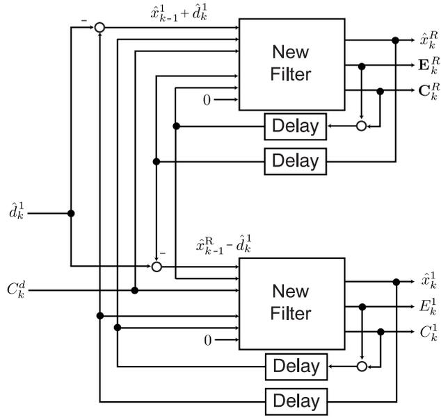
**Figure 1.** Block diagram of the algorithm for updating the position of wall 1 and the observer position with a measurement  $d_k^1$ . Please note, that the observer is assumed motionless for simplicity, which allows to omit the prediction step.
