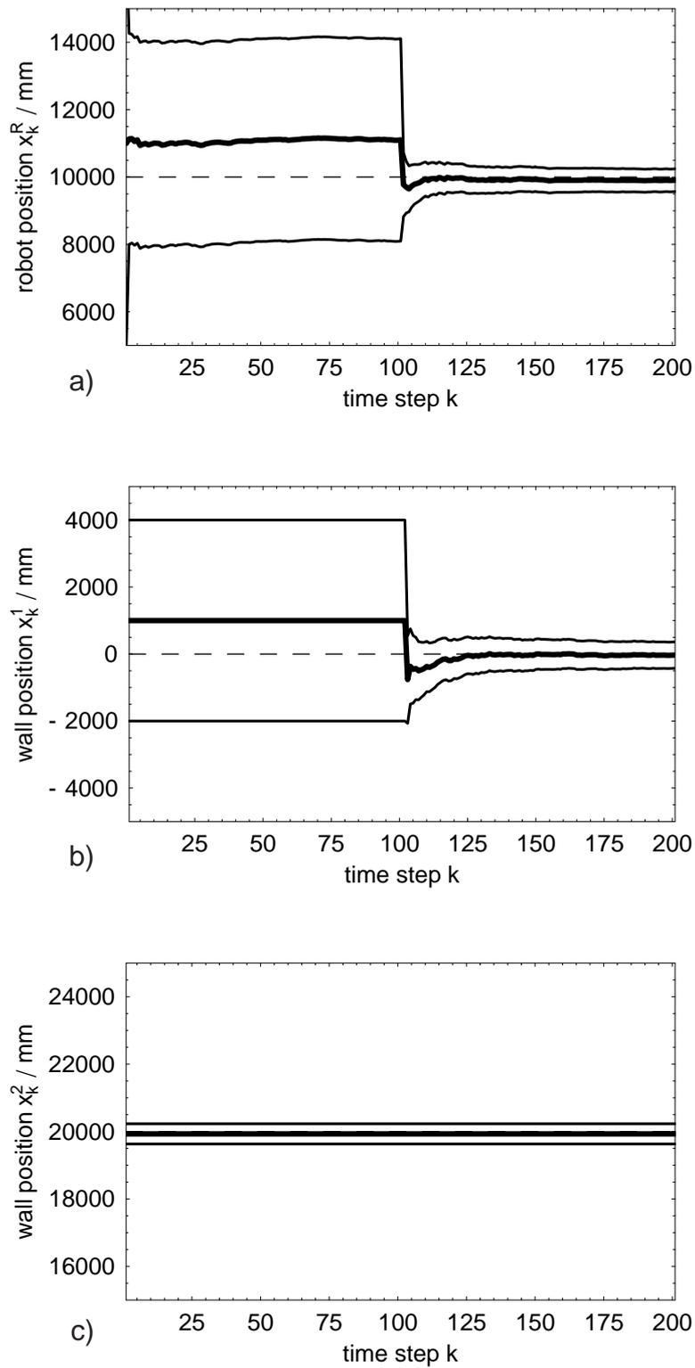
**Figure 5.** Results of applying the proposed new filter. a) Estimate of robot position. b) Estimate of position of wall 1. c) Estimate of position of wall 2. The figure shows the evolution of the estimated value (thick line) and the evolution of the  $3\sigma$ -bounds.
