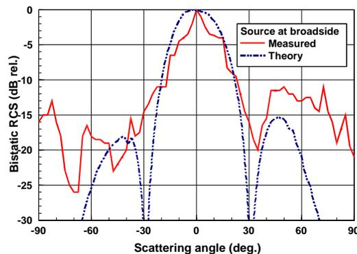
Fig. 6 Bistatic RCS, source at broadside (0°).
