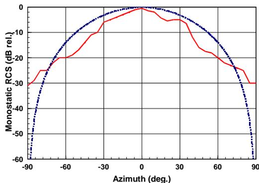
Fig. 5 Monostatic RCS pattern.
