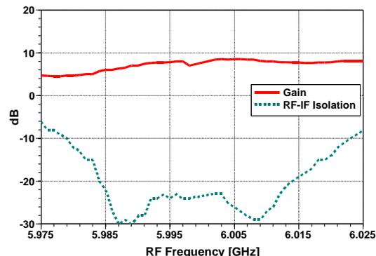
Fig. 3 Conversion gain and RF-IF isolation.
