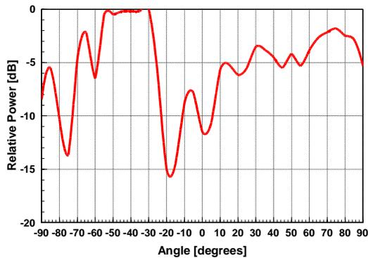
Fig. 12 Bistatic RCS, source at  $-30^\circ$ , RF= 5.8 GHz.
