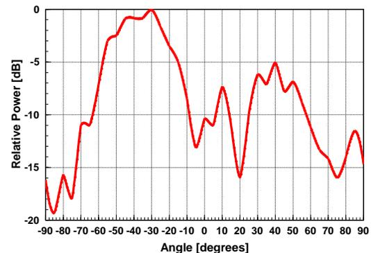
Fig. 11 Bistatic RCS, source at  $-30^\circ$ , RF= 5.2 GHz.
