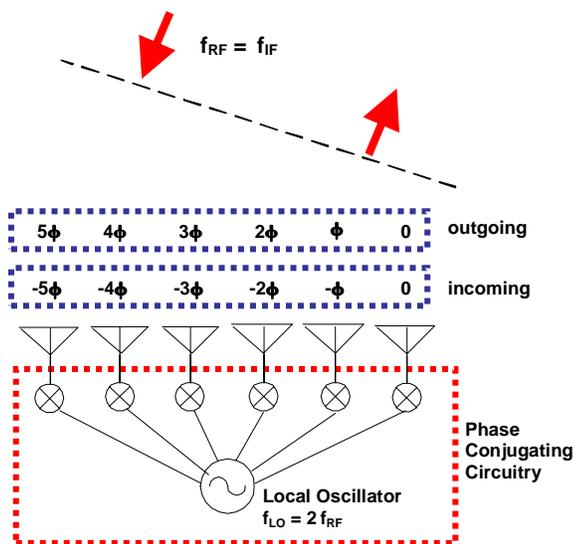
Fig. 1 Schematic of phase conjugating retrodirective array.
