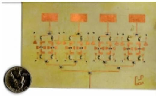
Fig. 4 Photo of the prototype 4-element active retrodirective array.
