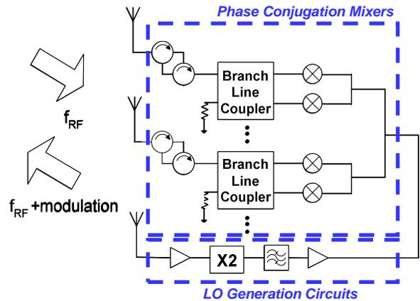
Fig. 10 Schematic of frequency autonomous retrodirective array.
