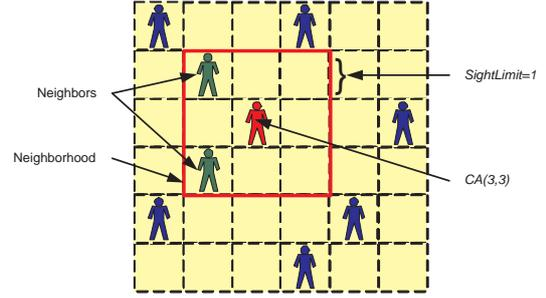
Figure 3: CA society distributed over a 2-d grid
