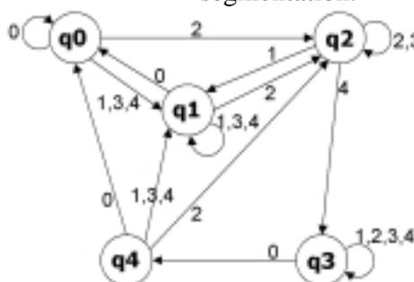
In this figure,  $q_0$ ,  $q_1$ ,  $q_2$ ,  $q_3$  and  $q_4$  mean 5 states, which are defined in Table 1, and arrows mean state transition functions and numbers on the arrow mean 5 motion phases such as ‘stop’, ‘preparation’, ‘stroke’, ‘moving’ and ‘end’ respectively, which are labeled as 0,1,2,3,4 respectively.
