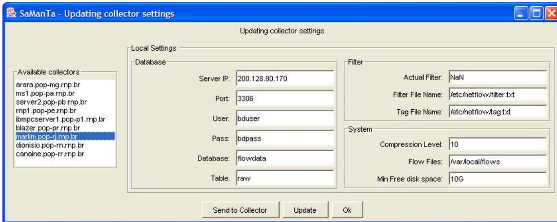
Fig. 8. Collectors configuration through SaManTa.
