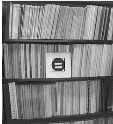
Figure 4: An artificial routemark. The square around the mark indicates that it has been recognized.
